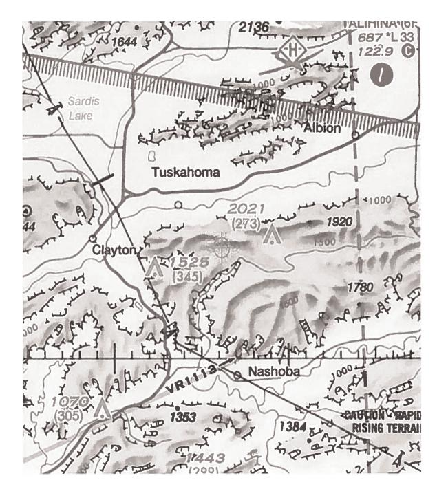
The proposed wind turbine is 1 of 70 wind turbines that would be located approximately 7.15 southeast through 1 1.96 nautical miles southwest of the Talihina Municipal Airport (6F1), Talihina, Oklahoma. The proposed turbine exceeds 14 CFR Part 77 Obstruction standards as described below.
