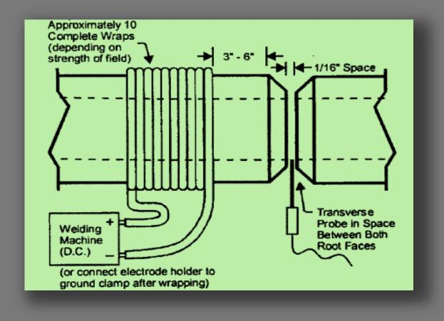
**NOTE:** On some projects, placing the coils one-half the diameter of the pipe from the joint to be welded reduced the field more than having the coil close to the joint.
