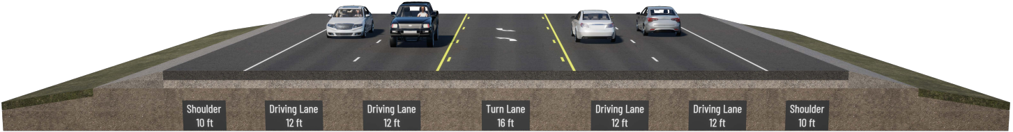
Typical Section 3 - 5-Lane Typical Roadway Section Includes four 12-foot-wide driving lanes with 10 foot-wide shoulders and a 16-foot-wide continuous left turn lane
