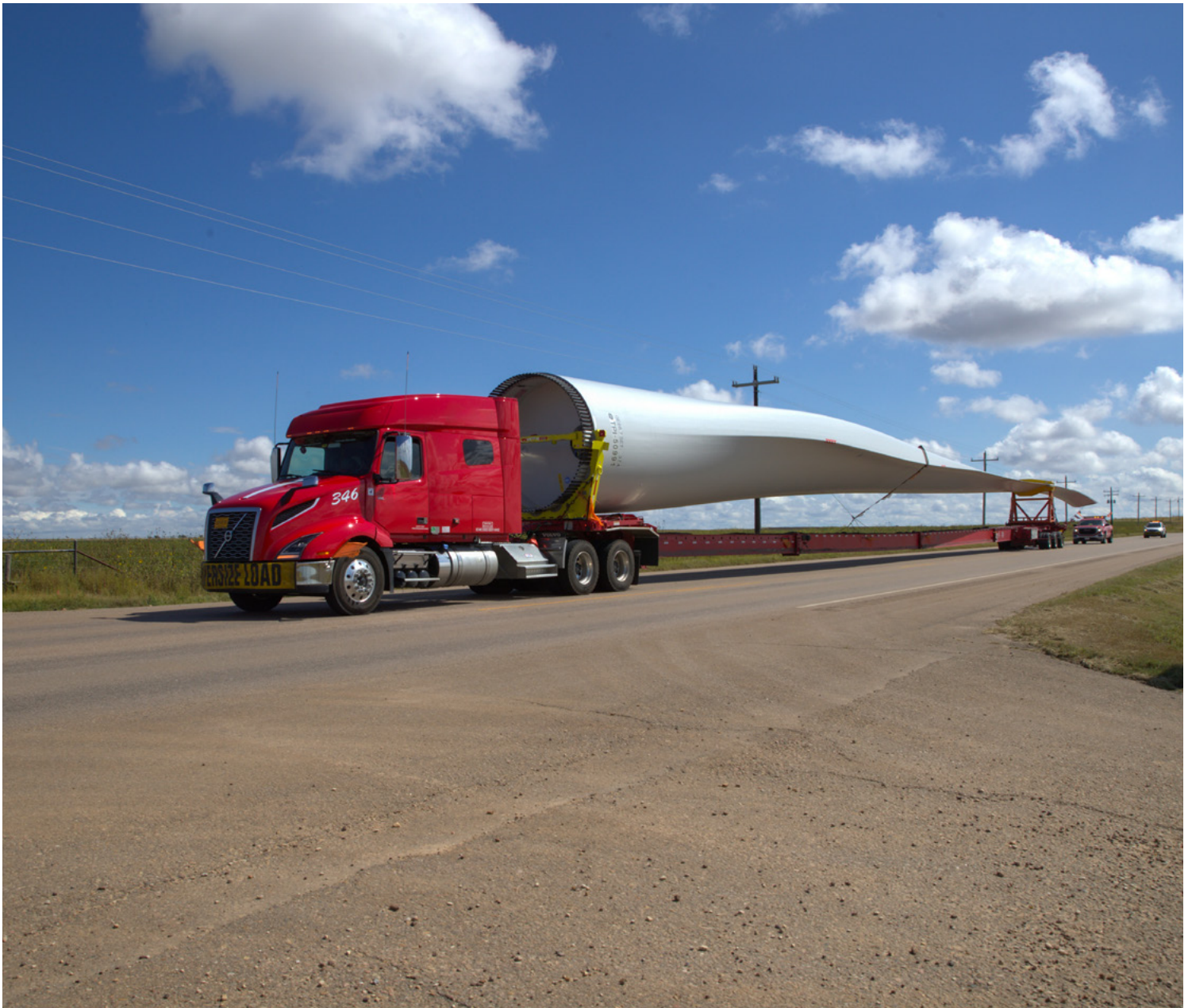
A blade of a wind turbine is transferred via semi-truck and specialized trailer with wide load safety flags and signs. Freight escorts follow in pick-ups with flashing lights.
