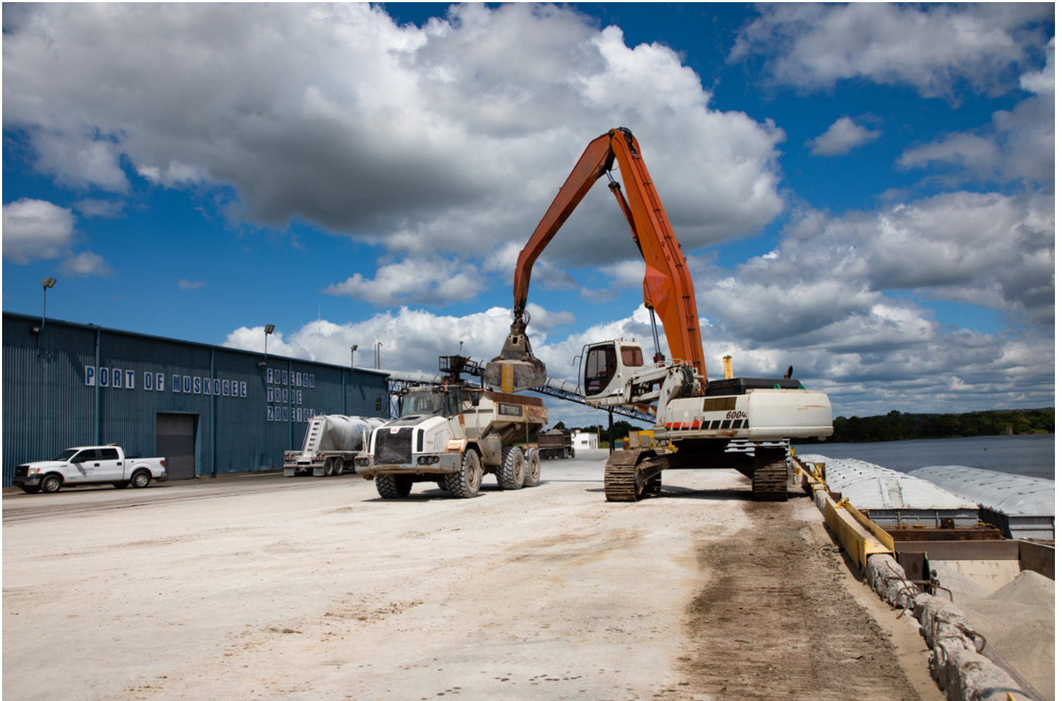
A material handler operator loads the back of a dump truck with sand-like material from a barge at the Port of Muskogee.
