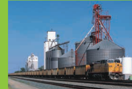
The Union Pacific Railroad connects Oklahoma's shortlines and major carriers to US markets west of the Mississippi. Its "unit train" approach uses 100+ cars to optimize fuel, car usage and destination options for the most economic means of transporting freight.
