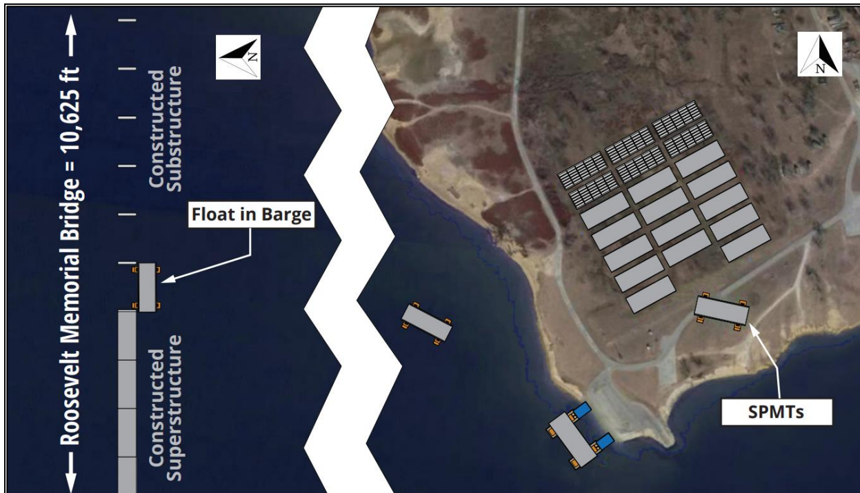
Figure 20: Illustration of a Float-in Modular Span Technique
