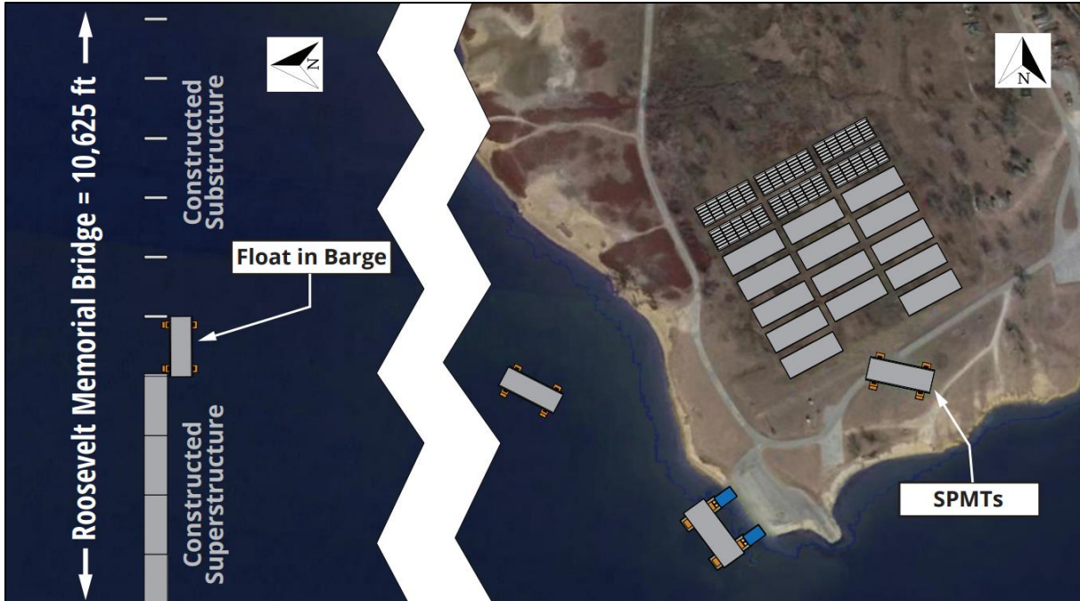
FIGURE 18: EXAMPLE OF A FLOAT-IN MODULAR SPAN TECHNIQUE
