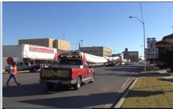
Flagger Truck stops approach to intersection at US-81/62.
