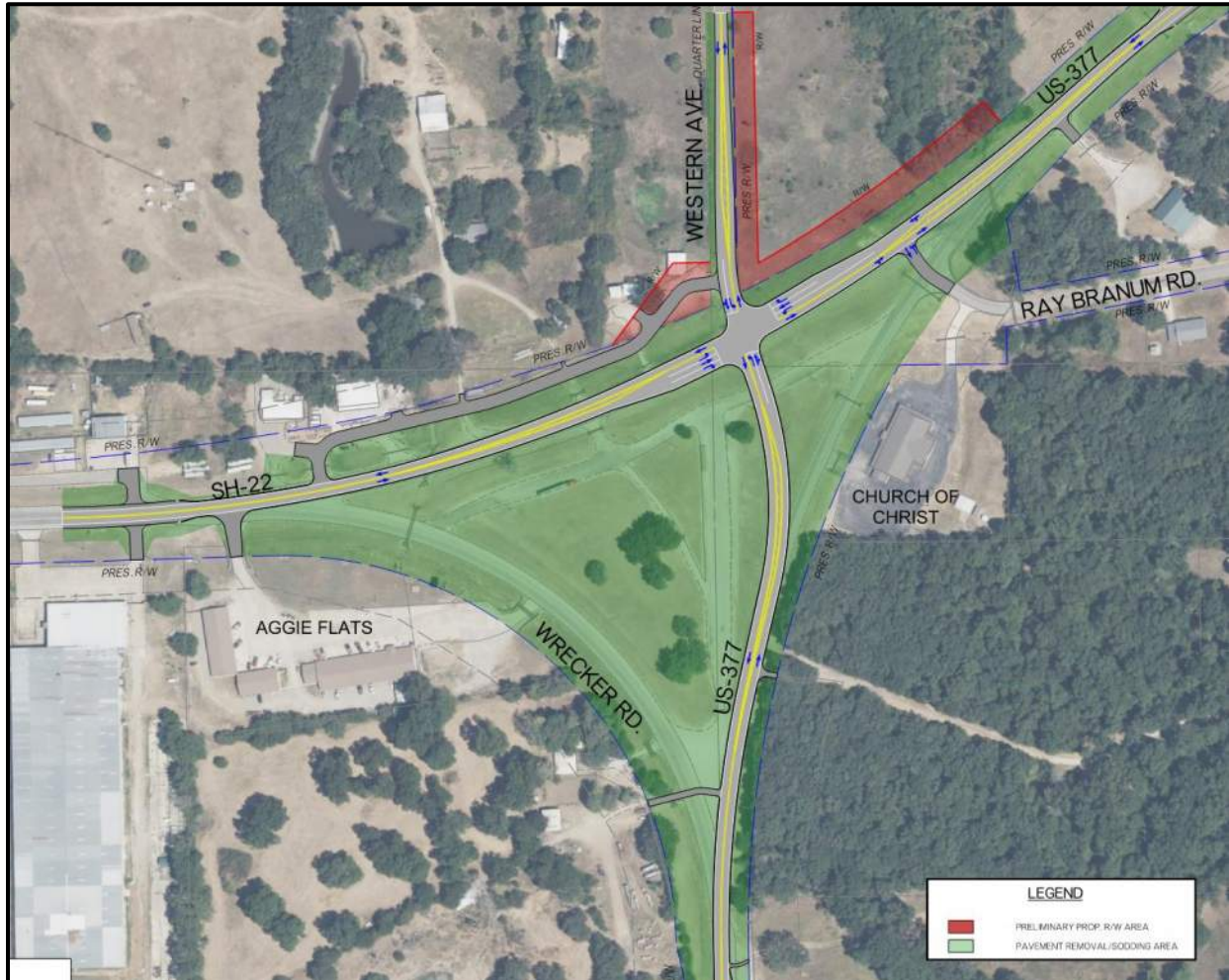
Figure 2 – Alternative 1 – Four-Legged Intersection
