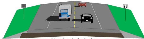
2-Lane Open Section Roadway Typical includes: two 12-foot wide driving lanes; 8-foot wide shoulders
