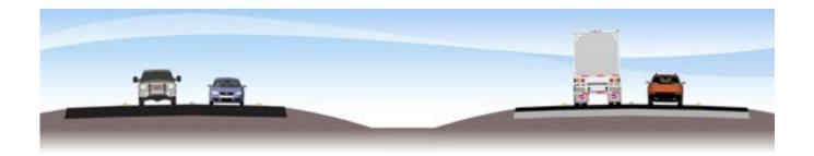
Typical section provides two 12-foot wide driving lanes in each direction with a 10-foot wide outside shoulder and a 4-foot wide inside shoulder with a variable 64 to 46 foot median.
