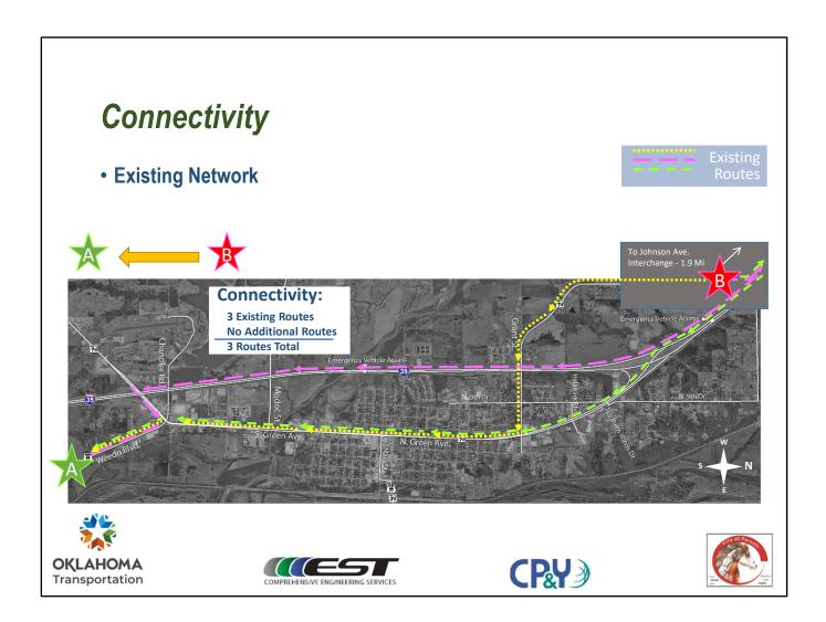
Again, the base line condition was determined finding the number of travel paths between Point B and Point A using the existing network. There are 3 routes between points B and A.
