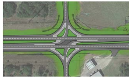
RCUT INTERSECTION ENLARGEMENT
