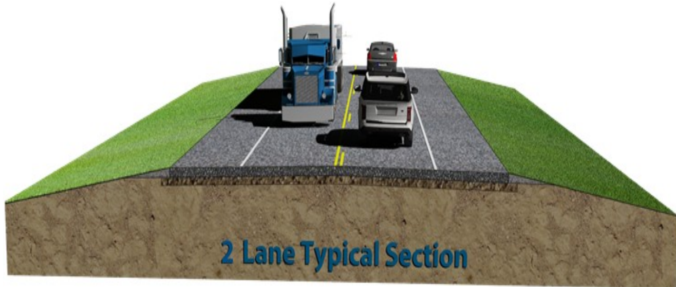
Typical includes: two 12-foot wide driving lanes and 8-foot wide paved shoulders, with 4-foot wide paved shoulders through Paradise Hill
