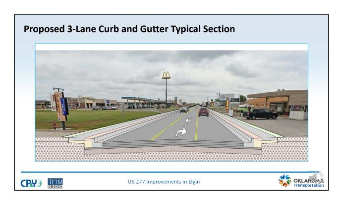
This image shows the proposed US-277 typical section, with one 12-foot driving lane in each direction, and a 12-foot continuous left turn lane, as well as curb and gutter and 4- to 6-foot sidewalks on both sides of the roadway.
