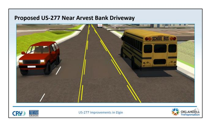
Pictured here is a rendering of the proposed project. A right turn lane is being introduced just east of Arvest Bank to accommodate traffic movements turning north onto the H.E. Bailey Turnpike. In most other locations, the roadway will consist of one 12-foot lane in each direction and a 12-foot two-way left turn lane.
