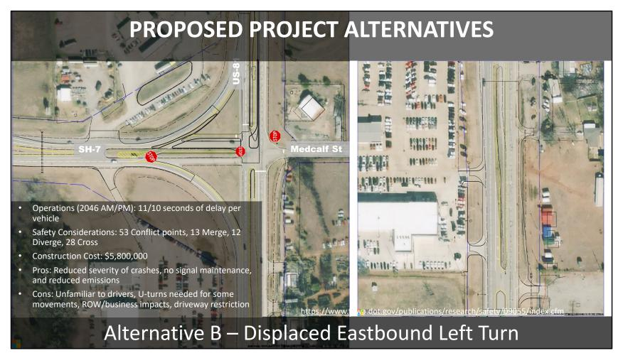
Another alternative being considered is Alternative B, which is a Displaced Eastbound to Northbound Left Turn. This alternative utilizes most of the existing pavement but does require some modifications.
