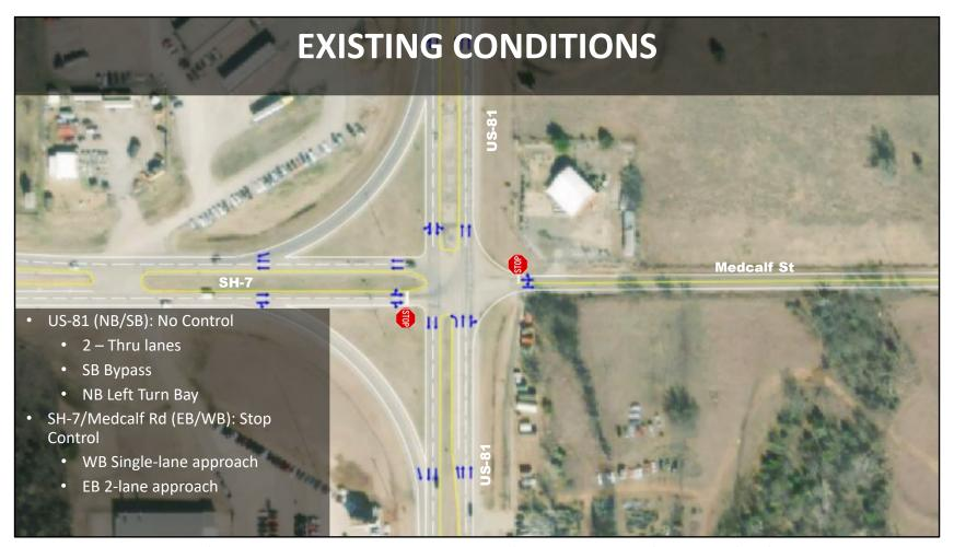
The existing intersection of US-81 and SH-7 is currently stop controlled for SH-7 and Medcalf Street and free flowing along US-81, northbound and southbound. Northbound US-81 provides a dedicated left-turn bay to SH-7 and two thru lanes, while the southbound US-81 approach provides two thru lanes with the innermost lane also serving left turns to Medcalf Street. Southbound US-81 provides a free flow right turn to SH-7 and eastbound SH-7 provides a free flow right turn to southbound US-81.
