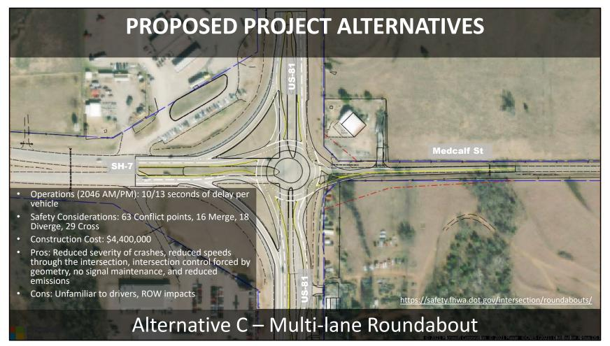
Alternative C is a Multi-lane Roundabout. This alternative utilizes curved approaches on US-81 to promote the slowing of traffic before entering the intersection. Provisions such as a truck apron around the center island and larger entry and exit radii, are provided to accommodate large vehicles like trucks, school buses, and emergency vehicles to navigate the intersection effectively.
