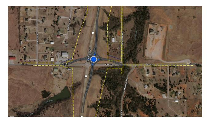
This roundabout is included as one of the alternatives to modify the existing intersection. The roundabout as shown in the conceptual drawing also has a total diameter of 162'-8", an apron width of 14', and a lane width of 16' and has been designed to allow a WB-67 truck to travel through with the trailer wheels tracking up on the apron. Right-turn bypass lanes have been added to the north side of the roundabout to improve the traffic operations based on the dominant turn movements.
