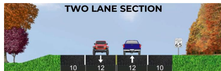
2-Lane Typical Roadway Section Typical includes: two 12-foot wide driving lanes; 10-foot wide shoulders
