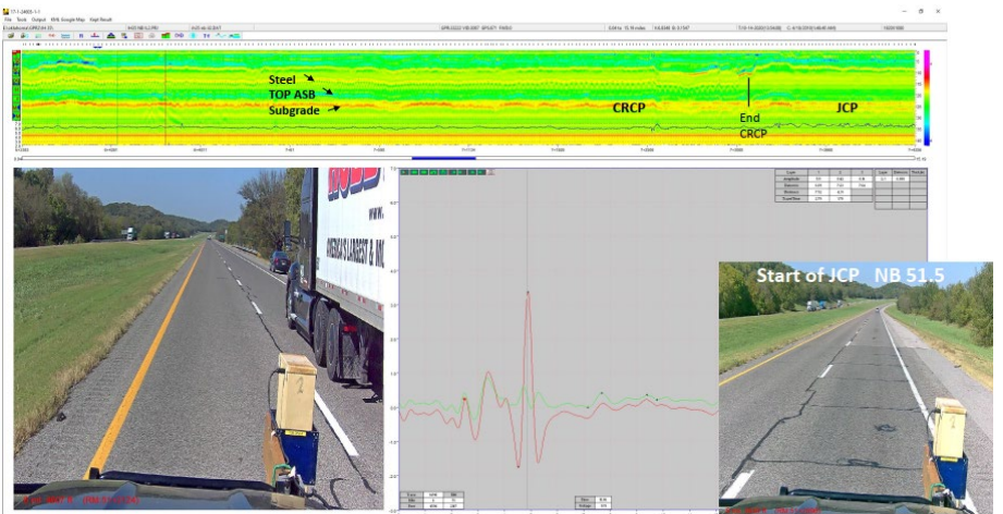
Figure 2 GPR and video images from north-bound I-35 section near Mile Post 51.5
