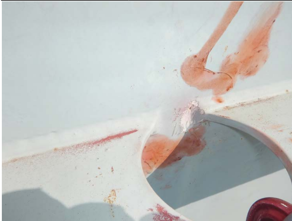
Photograph 3 - Looking north at span 5, girder 1 outboard between floor beams 4 and 5. Note: No MT indication.
