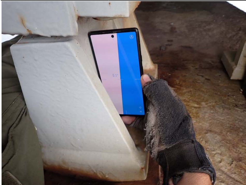
Photograph 72 - Looking north at the girder 1, span 10 expansion bearing at pier 10. Note: bearing is rocked 5 degrees in contraction at 77 F.
