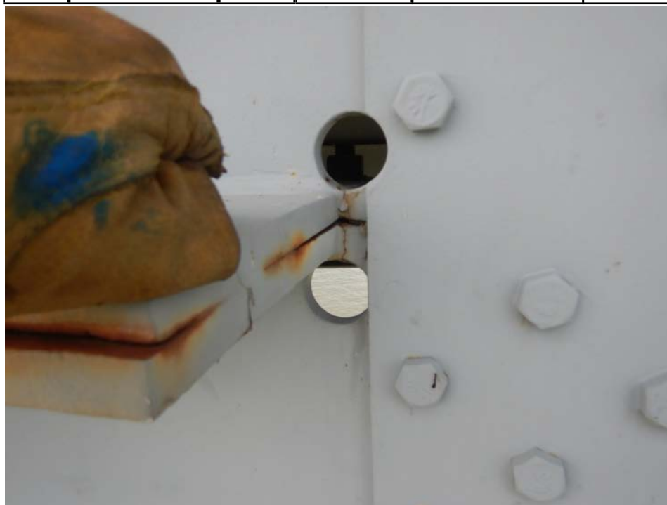
Photograph 22 - Looking north at girder 1, span 6 at the field splice near floor beam 3. Note: 3/4-inch-long crack in the inboard face at the horizontal web splice termination has not propagated past the arrestor holes.
