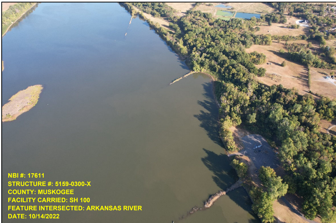
Photo 10 – Spur Dikes Along East Embankment Upstream of Bridge
