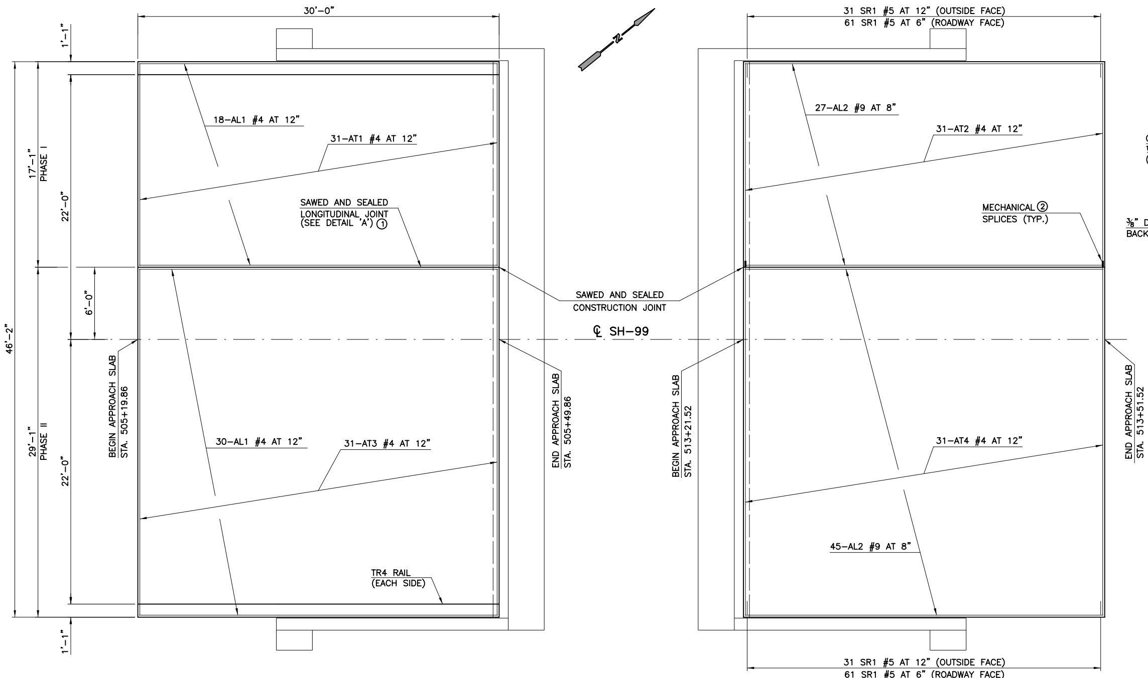
APPROACH SLAB NO. 1 TOP MAT OF REINFORCING STEEL SHOWN (TYPICAL FOR EACH APPROACH SLAB)
