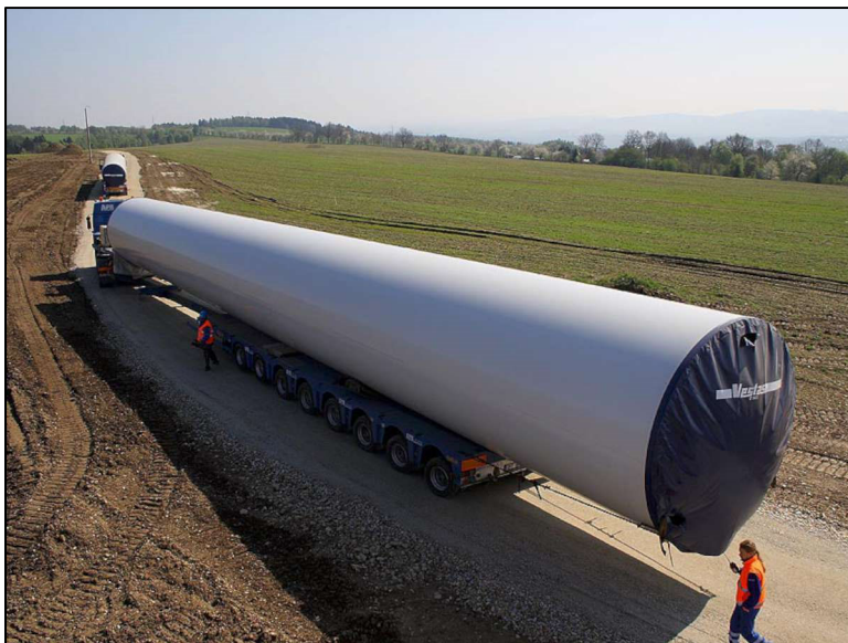
Figure 10: Transporting a Wind Turbine Tower Component
