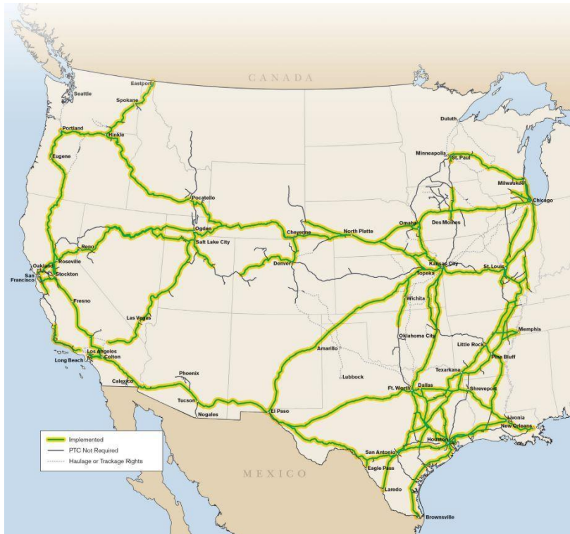
Figure 2-5: UP's PTC Implementation Source: Union Pacific 45 (As of December 2019)
