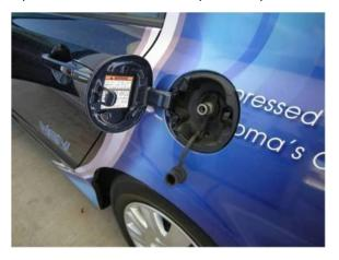
Note: Vehicles may have fueling adapters located in different areas, especially when they were converted to CNG i.e. under the hood.
