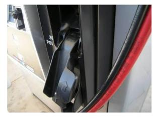
**Note:** During the fueling process you will hear the pump stop a few times, which will be accompanied with the hissing sound cycles. Fueling system is checking the pressure in the vehicle's tank(s).
