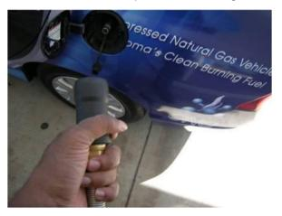
2.3.8. Check to ensure the nozzle is securely locked on the fuel adapter on the vehicle.
