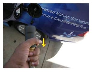
2.3.7. Push the nozzle to the quick-connect fitting on the vehicle.
