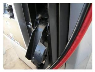
2.5.2. Turn lever on valve off. The pointed end of the valve should point away from the dispenser-end of the hose nozzle.
