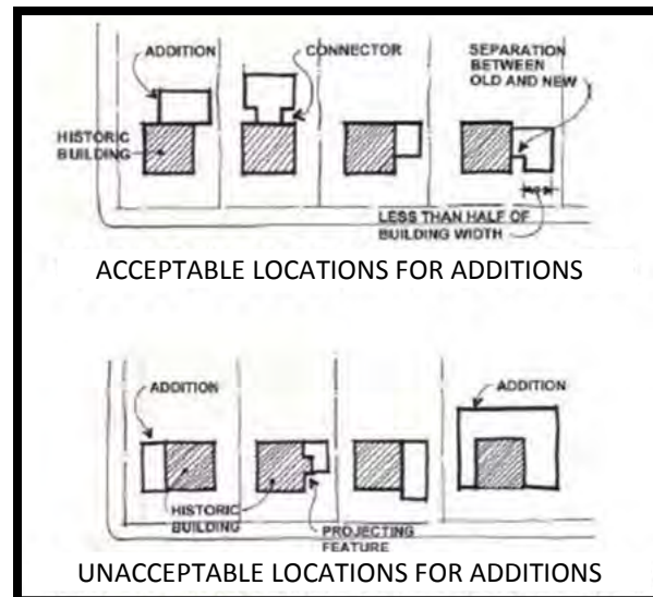
FIGURE 41: EXAMPLES OF ACCEPTABLE AND UNACCEPTABLE ADDITION LOCATIONS.
