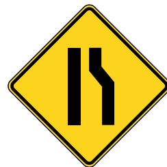
Right lane ends ahead. Prepare to merge.
